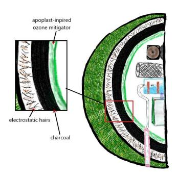
contains the radon-specific air filter, the VOC filter, and the "oxy-pro chamber." The radonspecific air filter targets radon, a very harmful pollutant, and clears it from the air. The VOC filter, inspired by poplar trees, has a series of actions. First, the VOC filter mimicks the poplar trees in absorbing a substantial amount of VOCs. The VOCs then reach a plasma catalytic converter that is located inside the filter where they are broken down. There are current air
