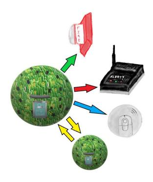
other systems. Under "Auto," the flag will be set as moderate under the circumstance of a laboratory leak or high pollutant ratio, and the device would only communicate with other systems. The flag will be set as severe under the scenario of a fire in which the device would stop oxygen production and then send an alert to systems. The "OFF" mode stops oxygen production completely, and to produce oxygen, the device would manually need to be turned to
